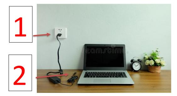
To Reduce the potential for a spark from the outlet, plug the cord into the wall and then into the device.
